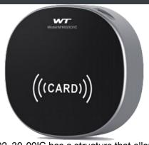
The WT-M-1602–30-00IC has a structure that allows the lock body to be turned after the card is read. The unlock light turns on after a card authorized to open has been read. You can open the lock body by turning it within 3 seconds. If you don't turn the lock body within 3 seconds, it will lock again. When the lock body is turned to the locked position while it is open, it is automatically locked.
