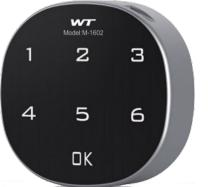
The WT-M-1602-30 has a structure that allows the lock body to be turned after the PIN is entered. The unlock light turns on after a PIN authorized to open is entered. You can open the lock body by turning it within 3 seconds. If you don't turn the lock body within 3 seconds, it will lock again. When the lock body is turned to the locked position while it is open, it is automatically locked.
